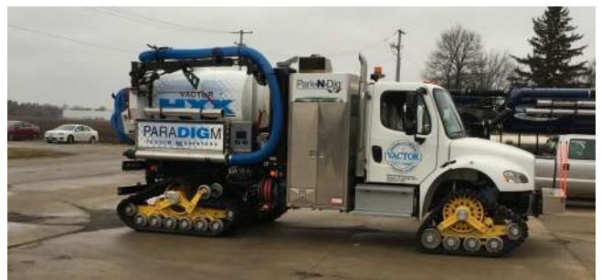
Figure 4. A Matracks 400M1A1 track conversion system on a Vactor HXX Paradigm Class 7 truck.
